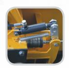
Mechanical system for constant lowering speed of the carriage.
