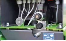
Speed of infeed adjustable by flow divider
