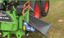
Infeed switch off due to saftey rope from steel
