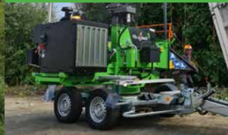
Massive turnable assembly 270° rotatable
