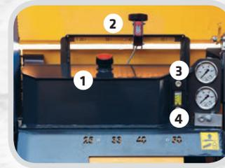
1. Oil tank for automatic chain lubrication with an oil level indicator.
