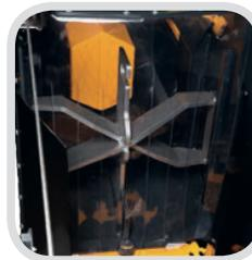
Hydraulically adjustable height of the splitting knife
