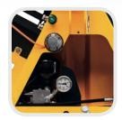
Pressure relief brake for constant tension of the wire rope on the drum.
