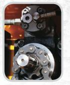
Hydraulic pump is gear driven.
