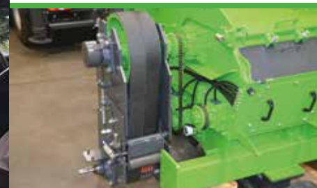
Massive V-belt transmission
