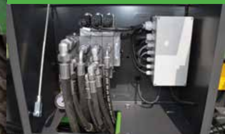
Hydraulic control block
