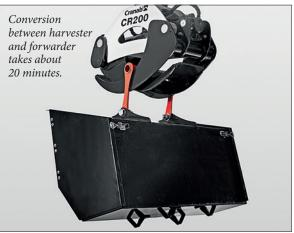
Stand-operative dual machine which simply and easily converts between harvester and forwarder without compromising productivity or performance. A unique solution with removable counterweights allows the Combi to perform as well as a traditional harvester.
