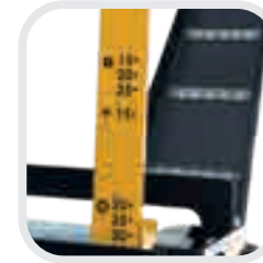
Splitting knife height regulation in correlation with nr. of logs and log diameter.
