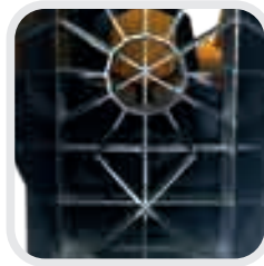
One multilevel hydraulically adjustable 2-4-8-18-way splitting knife.
