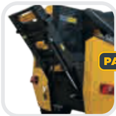
Built-in hydraulically foldable feed-in table.
