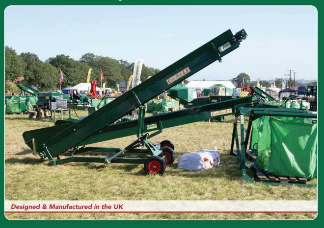
This 4.5 metre adjustable and portable conveyor enables the easy loading of firewood into bags or vehicles. Reduces manual handling and increases productivity. Single person operation with wide positioned wheels that makes the conveyor easy and safe to move around. The conveyor can be adjusted to a very low height making it suitable to move large rings without the danger of them rolling down if the conveyor is at a steep angle. Supplied with swivel / braked wheels as standard.
