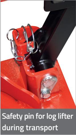
Safety pin for log lifter during transport
