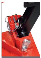
Safety pin for log lifter during transport
