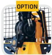
AUTO STOP function (limit switch) automatically stops the function of winding the wire rope on the drum. This function prevents mechanical damages of the unwinding device, entanglement and wire rope damages.
