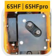
Winches 65HF and 65HFpro can be installed at front or rear. Both models have unwinding device as standard equipment.
