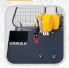
Plenty of room for forestry chains and other small forestry accessories on the front side of the butt plate to prevent the dirt from entering the chains and other equipment.
